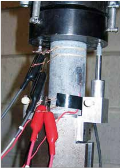
► Figure 7 Smart concrete; Left: sensor in compression; Right: sensor in tension
