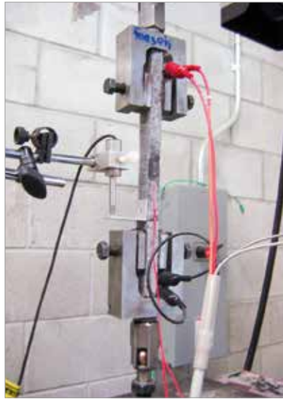
► Figure 7 Smart concrete; Left: sensor in compression; Right: sensor in tension
