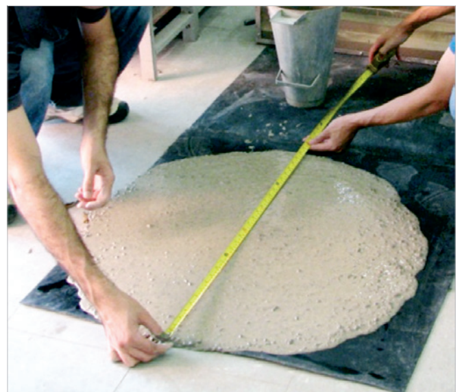
Figura 5 – Slump flow diameter measurement
