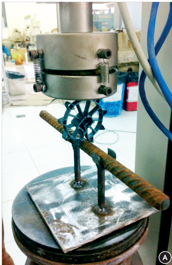
Figure 14 – Spacer application test to the steel bar: a) in circular spacers; b) in chair-type spacers
