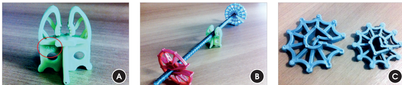
Figure 3 – Explanation of the identification requirement: a) size of the covering on the product; (b) separate colors between spacers with different coverings; c) spacer from the same manufacturer, of the same type and the same model, but with different coverings
