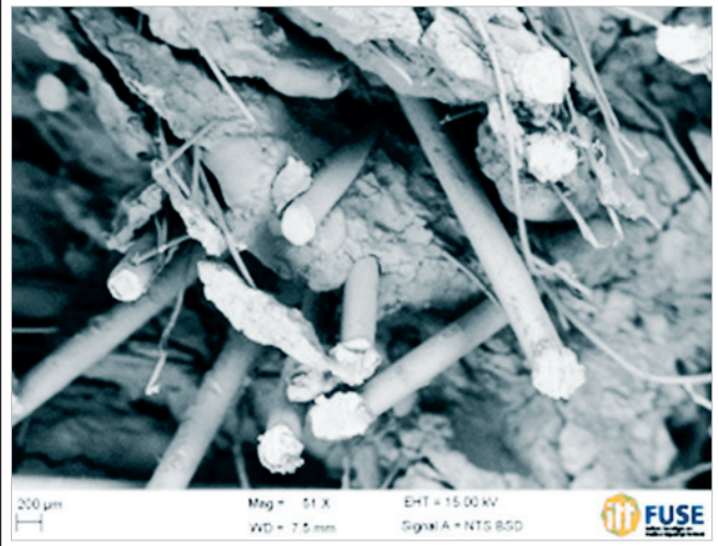
Figure 11 – SEM image of the distribution and geometry of the fibers in a sample stretch
