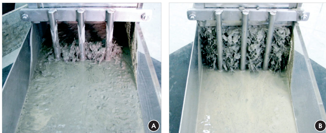
Figure 7 – Aspect of the L-Box after the test for the fiber contents of 80 kg/m 3 (a) and 120 kg/m 3 (b)
