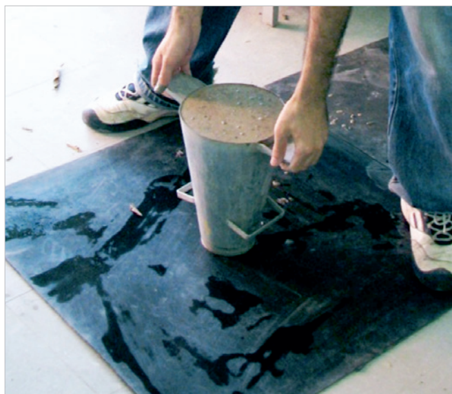
Figura 5 – Slump flow diameter measurement
