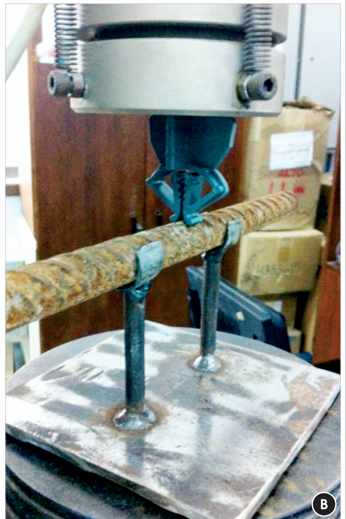
Figure 14 – Spacer application test to the steel bar: a) in circular spacers; b) in chair-type spacers
