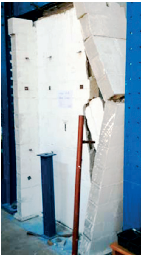
Figure 15 - Failure - flanged wall without central support 04
