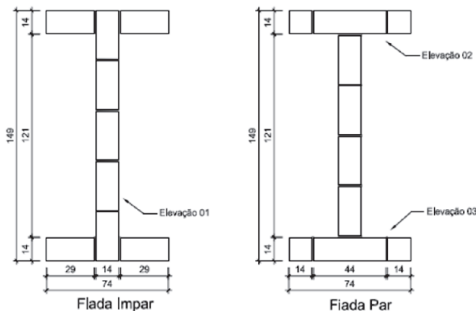
Figure 1 – Dimensions of flanged walls on site. 260 cm height walls | Heights in cm
