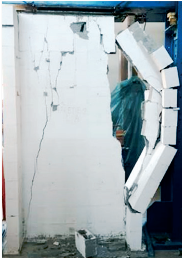
Figure 13 - Failure - flanged wall with central support 02
