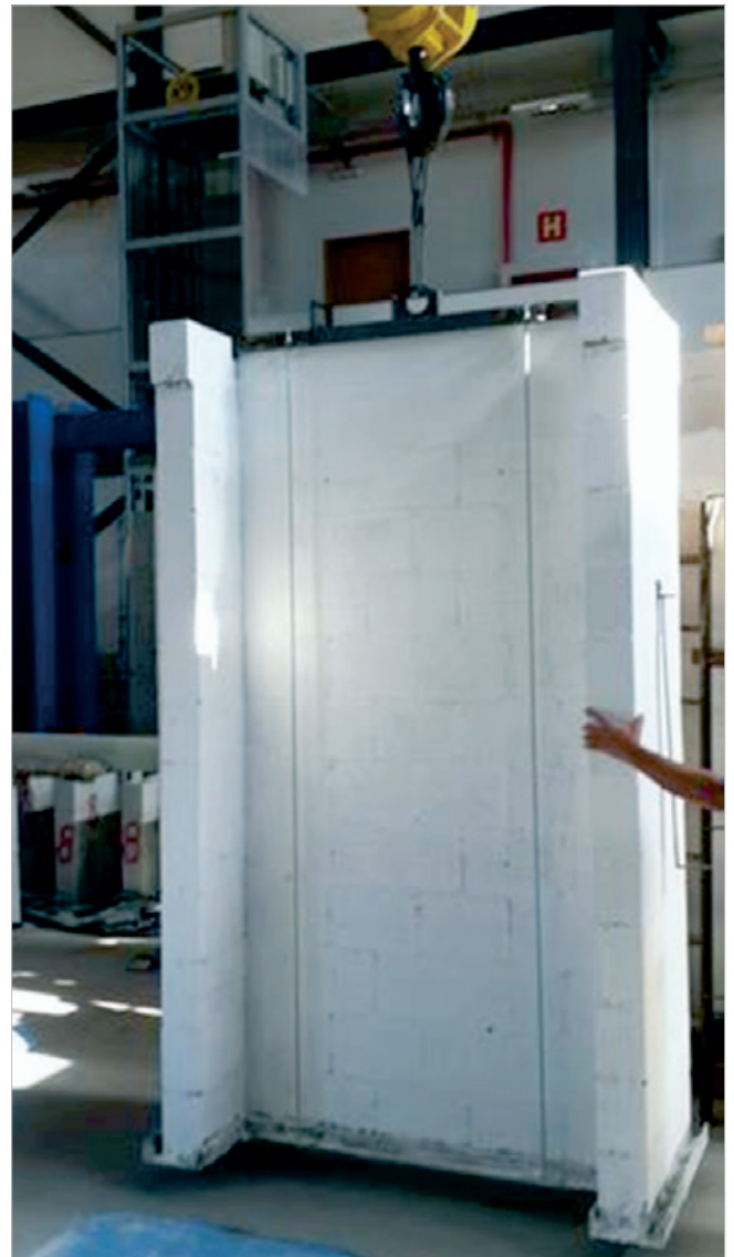
Figure 3 – Executed flanged wall and its transportation to the reaction portico by rolling bridge
