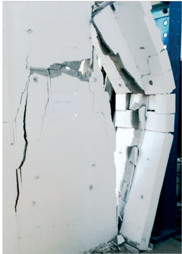
Figure 12 - Failure - flanged wall with central support 01
