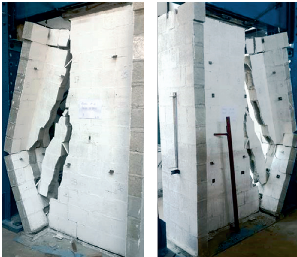
Figure 17 - Failure - flanged wall without central support 06
