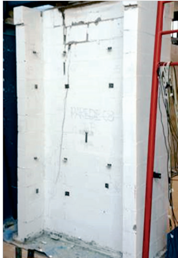
Figure 14 - Failure - flanged wall with central support 03
