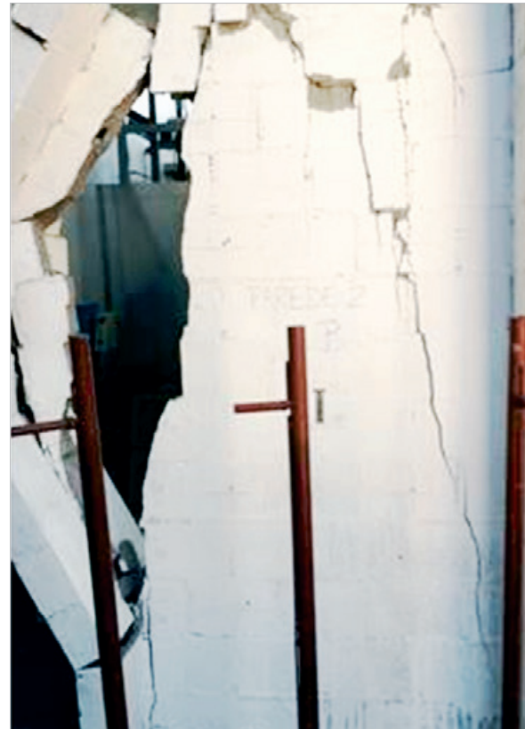
Figure 13 - Failure - flanged wall with central support 02
