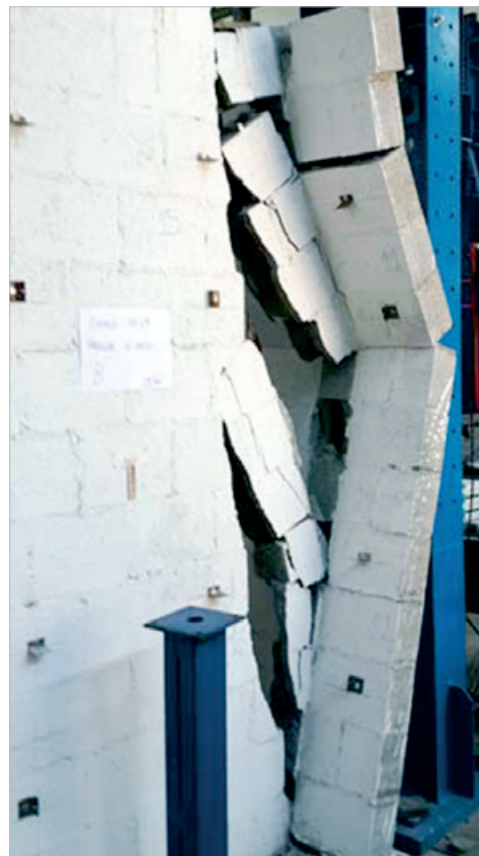
Figure 15 - Failure - flanged wall without central support 04
