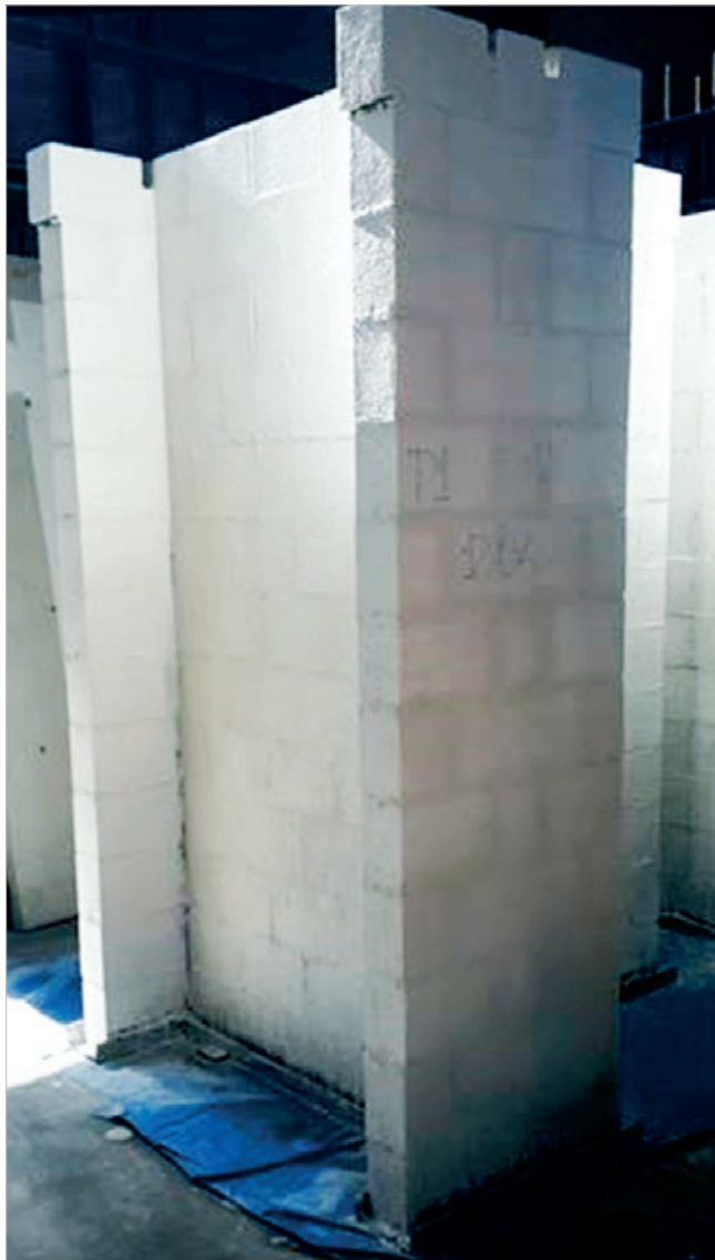
Figure 3 – Executed flanged wall and its transportation to the reaction portico by rolling bridge
