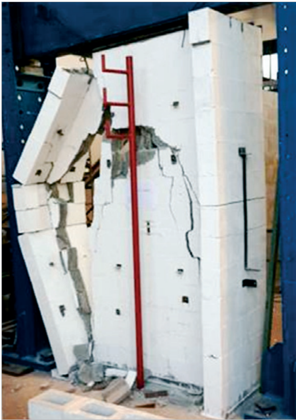
Figure 12 - Failure - flanged wall with central support 01
