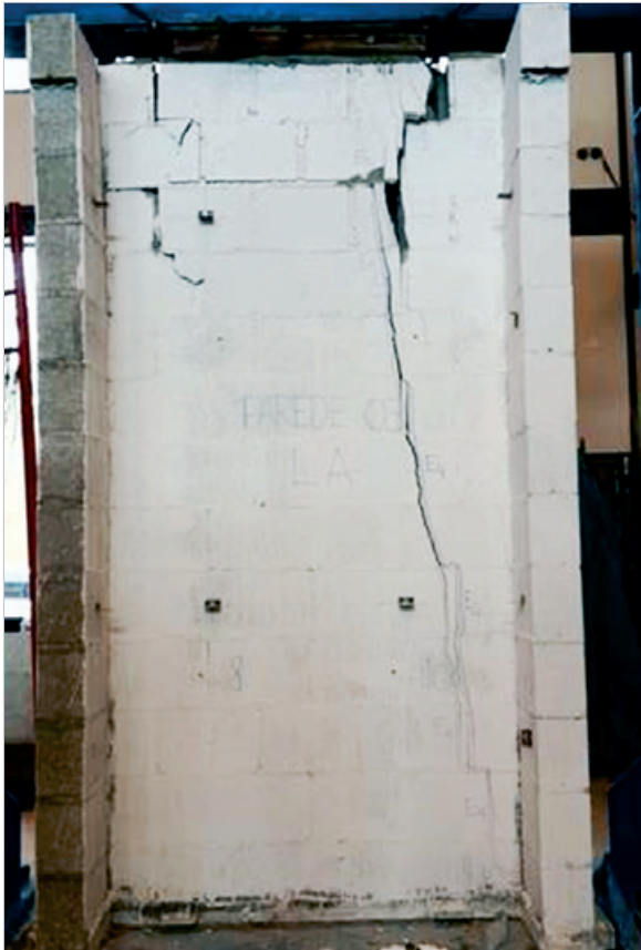
Figure 14 - Failure - flanged wall with central support 03
