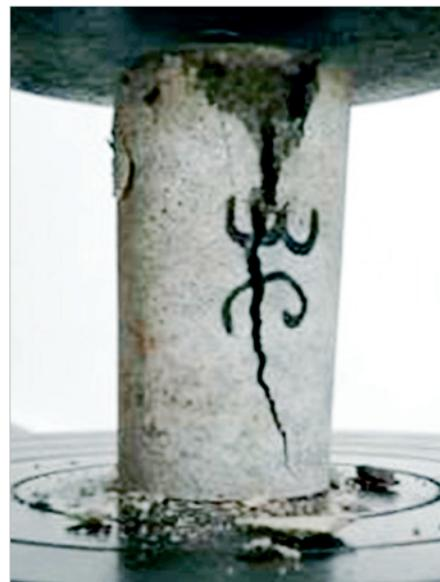
A Shear plane mode of failure
