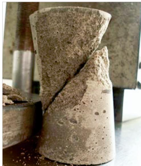
cylindrical (48.01%, 44.07% and 36.83%, respectively). This means that the effects related to the ends of the specimens (present in the cylindrical ones) have influenced the results, while results for the specimens in the hourglass shape represent only the determination of the resistance of the material. Thus, the measurement of the characteristic 'strength of con-
