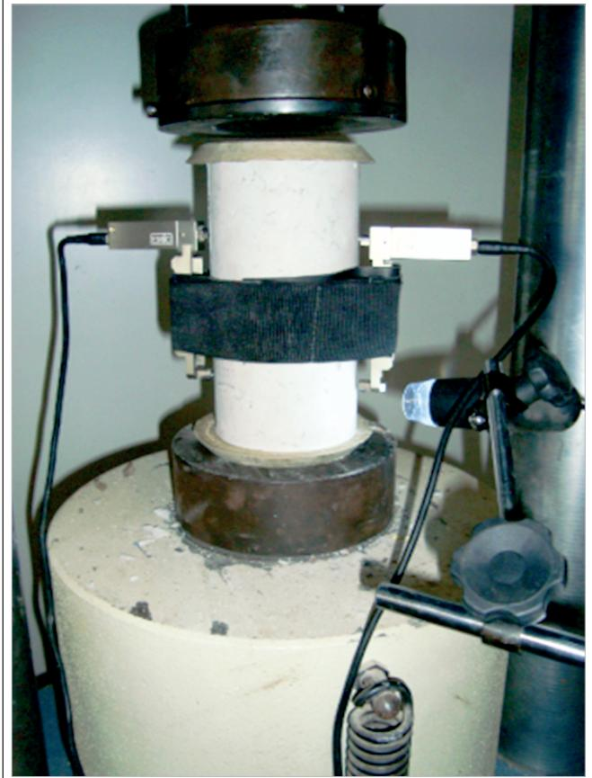
Loading and unloading cycles were performed to stabilize the test at a rate of 0.45 MPa/s for intervals of 30 seconds between loading and unloading.
