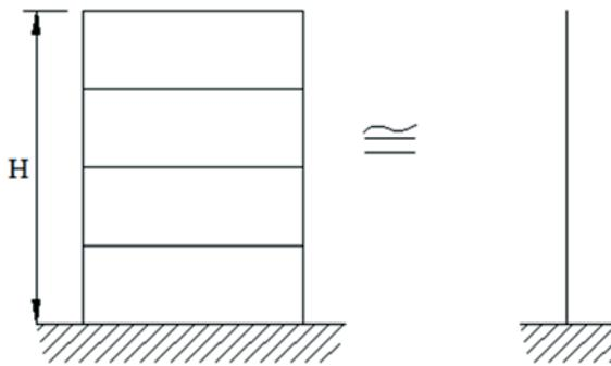
is performed by the Stability parameter  $\alpha$ . Above a certain limit value, the structure is classified as of mobile nodes, and therefore should be considered second-order analysis. It is emphasized that the parameter is not able to estimate the effects of second order.
