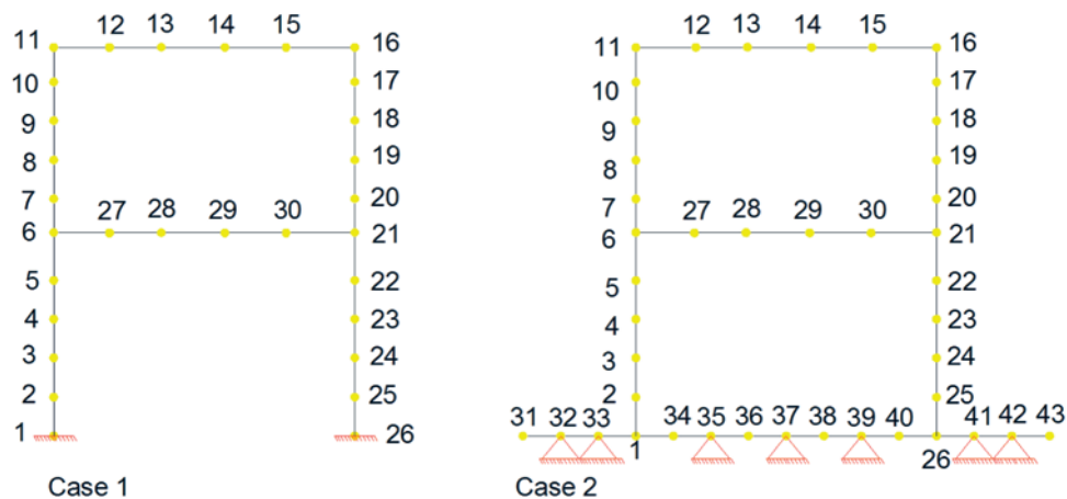
Figure 12 – Mesh and Boundary conditions used for the analyses
