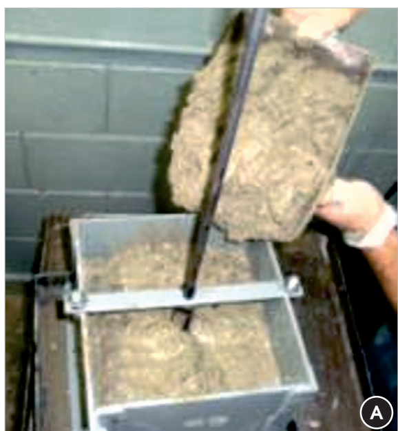
Figure 8 - Concreting in metallic mold on a vibrating table (a); specimens POT concreted (b)
