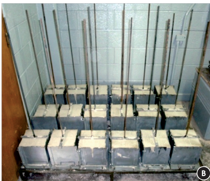
Figure 8 - Concreting in metallic mold on a vibrating table (a); specimens POT concreted (b)
