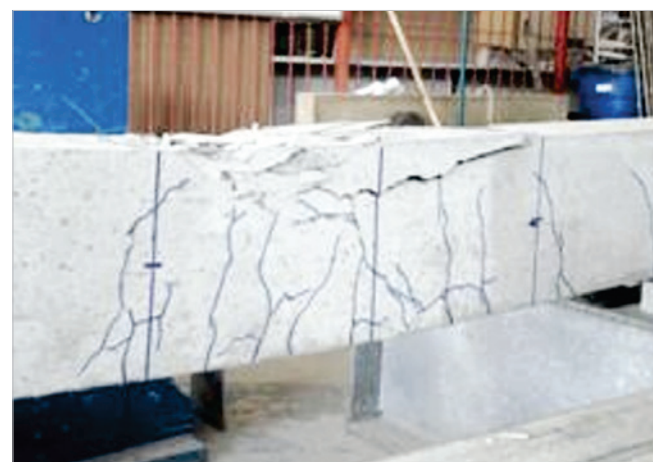
Figure 8 State of the beams after the experiments. (a) Geopolymer concrete (b) Portland concrete
