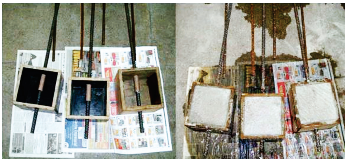
Figure 5 Concreting direction of the prismatic models
