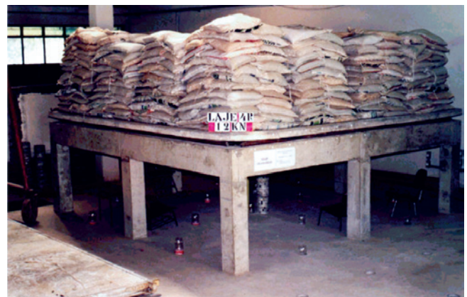
Figure 4 Slab L4R loaded of 12,0 kN/m 2
