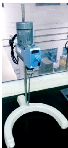
Figure 3.2 Mechanical stirrer IKA RW20 (left) and mixing conditions (right)
