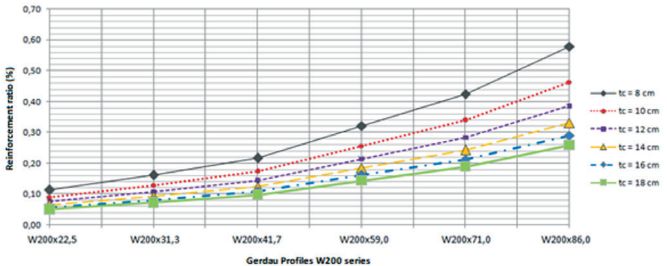
Figure 9 Reinforcement ratio x analyzed Gerdaul profile, W200 series
