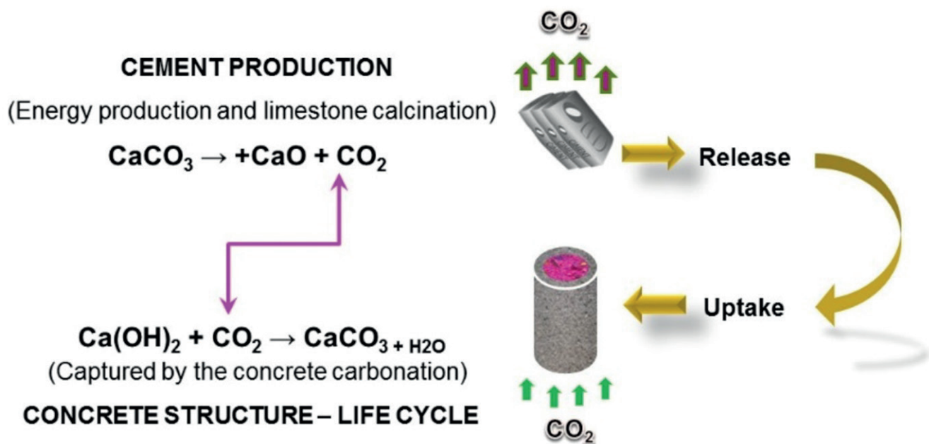
Figure 1 Concrete carbonation versus CO 2 uptake [23]
