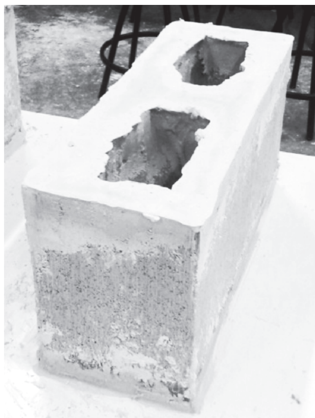
Figure 2 Block with plaster capping
