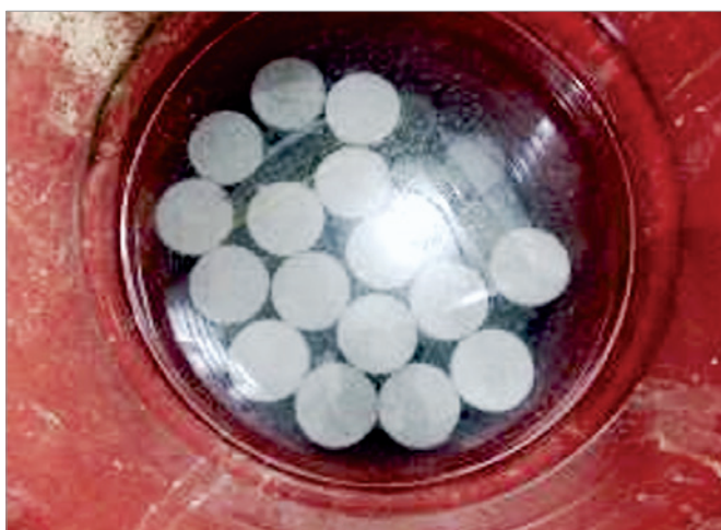
Figure 4 Grout specimens and grouted mid-height bond beam
