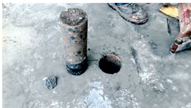
Figure 4 Forensic extraction of CRCP slab specimen
