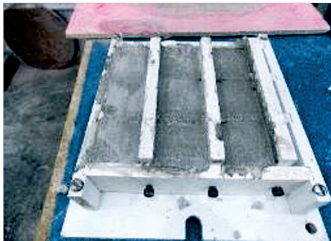
Figure 3 Prismatic mortar molding
