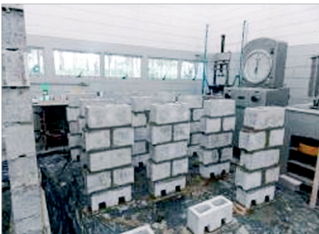
Figure 6 Hollow and grouted prism
