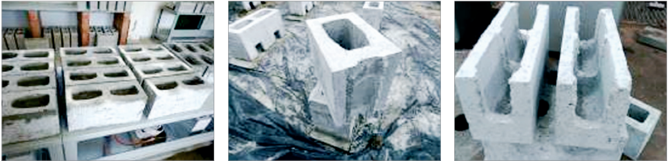
Figure 5 Standard concrete block, cut half-block; bond-beam block
