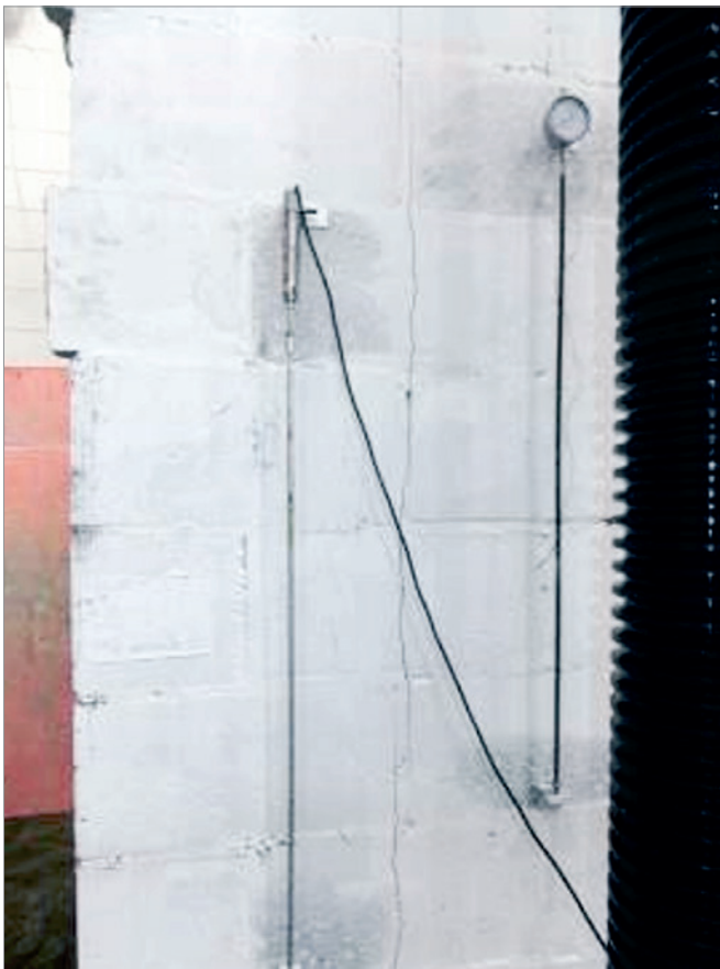
Figure 28 Hollow wall failure
