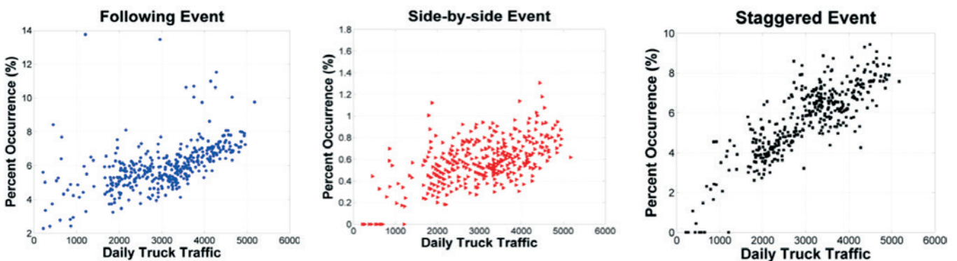
Figure 13 Variation of multiple presence for truck volumes (85.3-m span)
