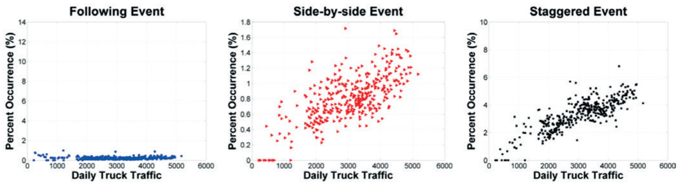
Figure 11 Variation of multiple presence for truck volumes (36.6-m span)
