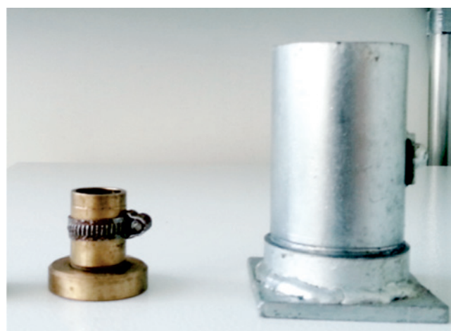
Figure 1 Specimen molds – (2x4) cm and (5x10) cm
