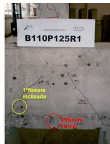
Initial cracks visible in the lower part of the block
