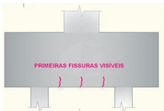
Initial cracks visible in the lower part of the block
