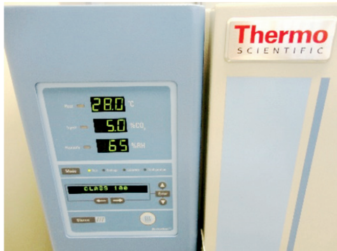
Figure 2 Carbonation chamber – exposure conditions of the specimens
