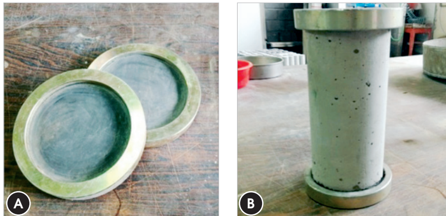
Figure 2 a) Retaining rings and neoprene pads; b) Specimen with neoprene caps
