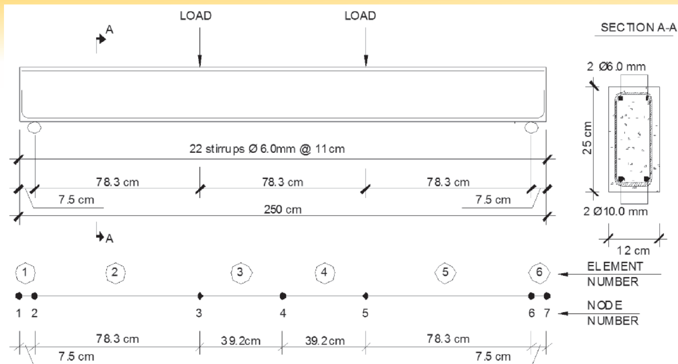
Figure 3 Tested beams (VT1 and VT2) geometry and reinforcement; load application and support positions (Beber (29))
