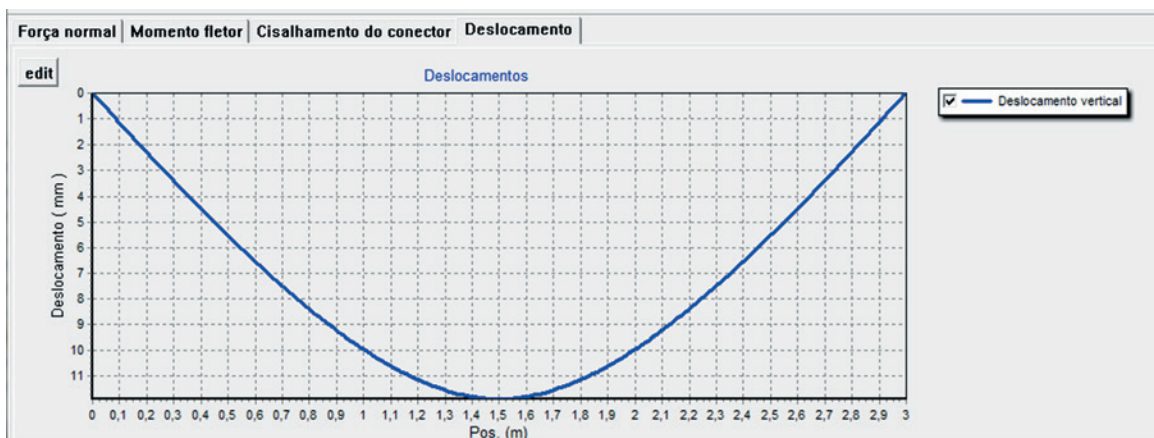
Figure 11 - Graph of vertical displacement along the length of the beam for the applied force of P_k = 15 \text{ kN}
