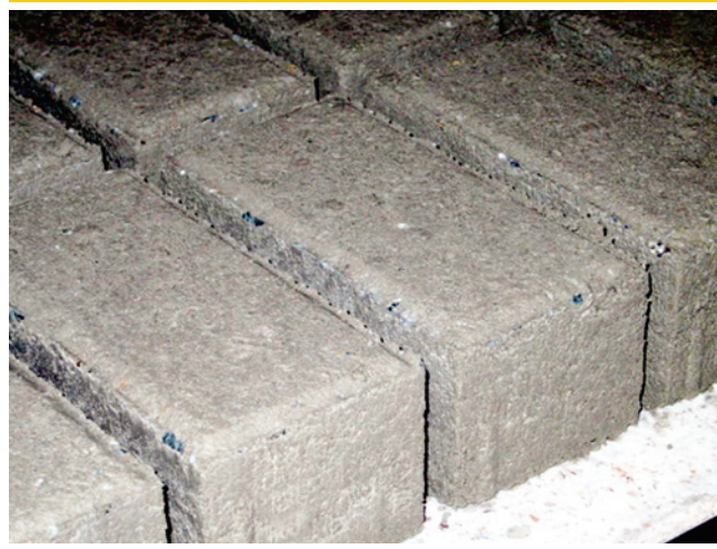
Figure 4 – Conventional Paver 8 concrete blocks
