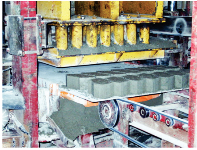
Figure 5 – Vibropress used in the production of the concrete blocks
