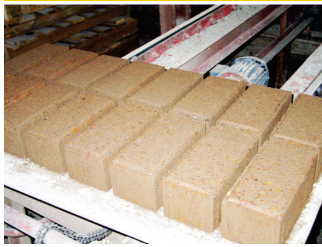
Figure 9 – Paver 8 blocks produced with sinter feed tailings
