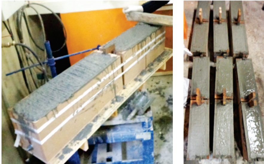
Figure 2 - concrete placement set beams for testing adherence between the bars and the concrete
