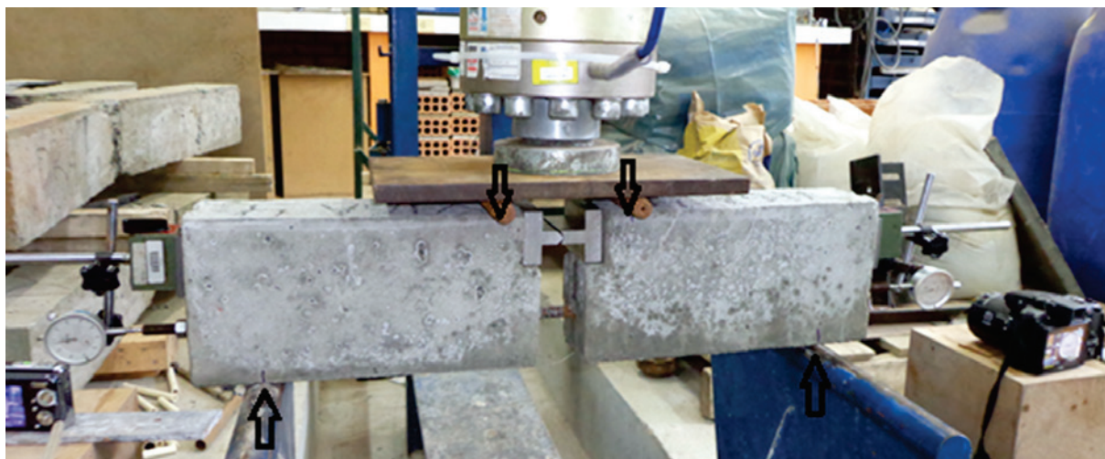
Figure 3 - Execution of the beam test
