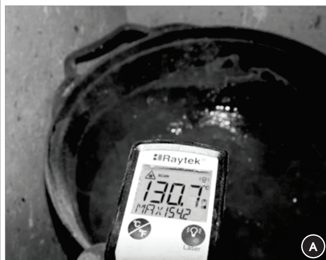
Figure 3 – Temperature of the sulfur mixture (A) (left) and capping of test specimen (B)
