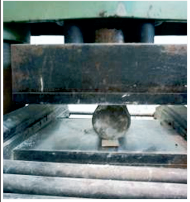
Figure 13 - Splitting tensile strength test by diametrical compression
