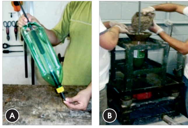
Figure 4 – (a) PET bottle mold (b) Concreting of the PET bottle mold on the metal support
