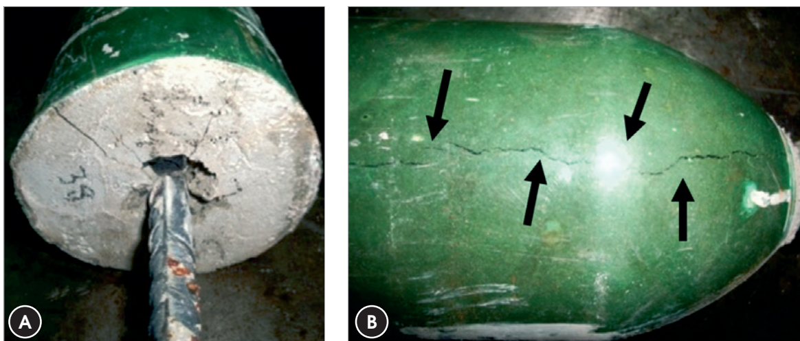
Figure 8 – Type of rupture by concrete splitting in the APULOT method with PET mold. (a) front view and (b) side view of test specimens
