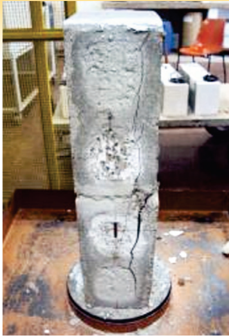
Figure 13 Lateral prism after testing
