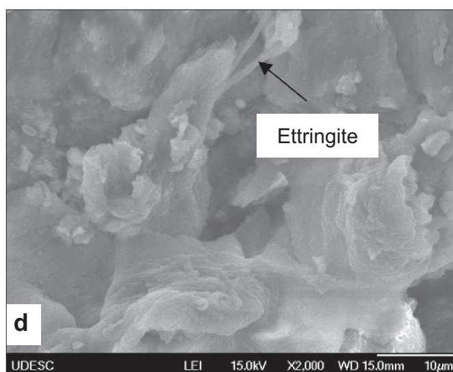
Figure 7 Mortar micrography, (a) formation of C-S-H, (c) formation of calcium hydroxide (CH), (c) rubber particles, (d) formation of late ettringite crystals ( C_6ASH_{31} )
