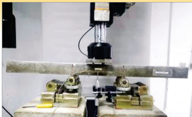
Figure 10 Beam before bending test (Author)
