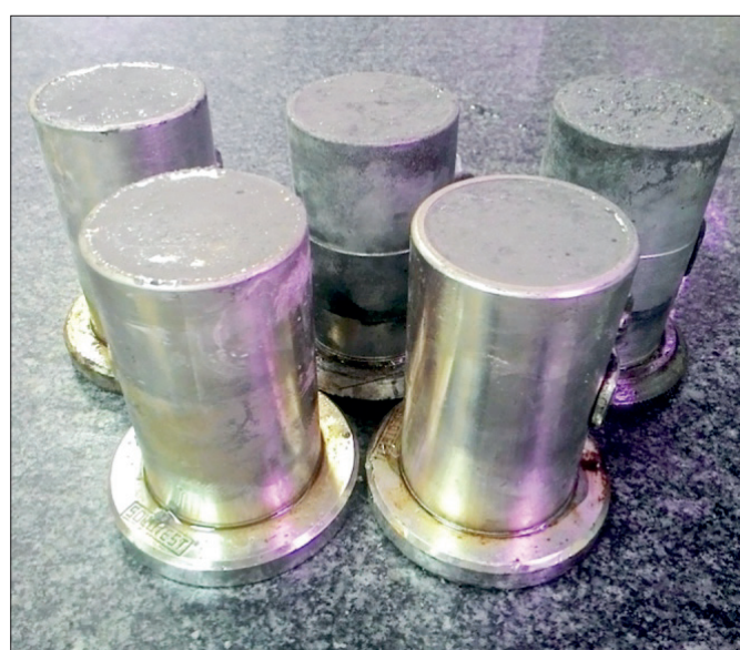
Figure 3 Specimens for pozzolanic activity
