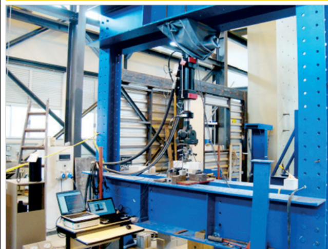
Figure 5 – Load application system – Frame with MTS 244.22 actuator
