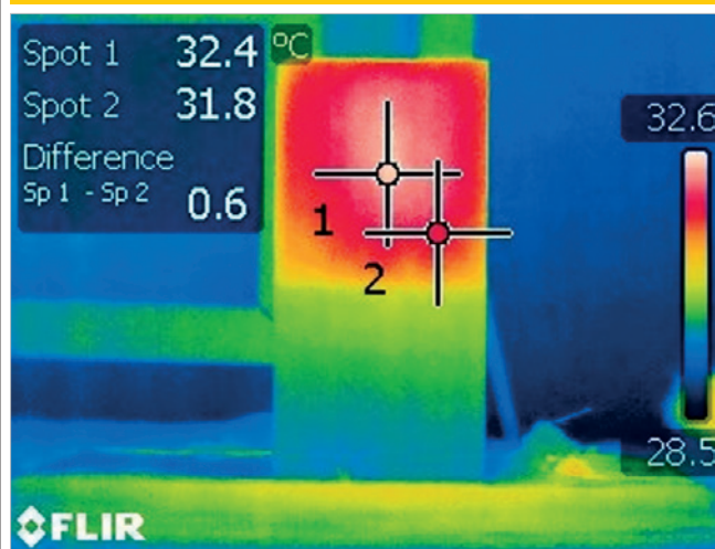
Figure 4 – CP1, group 1, complete adherence, heated by incandescent lamp
