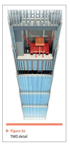
criteria compared to office buildings. Taking the steps above ensured occupancy comfort for different return periods. Building response was closely monitored during the construction to ensure Tuned Mass Damper will perform within the design range.
