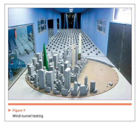
Comprehensive and projectspecific wind tunnel tests were performed at the Rowan Williams & Irvin (RWDI) wind tunnel facilities to determine more accurate wind loading and wind response of the tower with respect to human comfort criteria.
