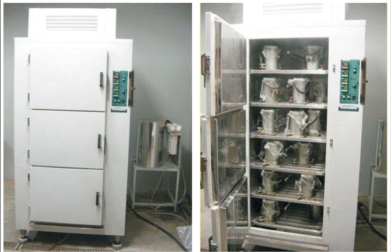
Figure 2 – Steam curing equipment
