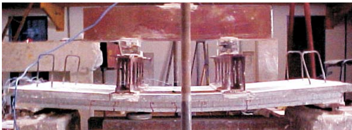
Figure 6 – Typical slab at failure
