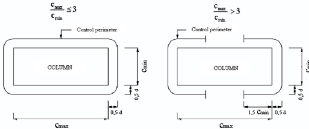
Figure 3 – Control perimeter according to NBR 6118:2003 code (2)
