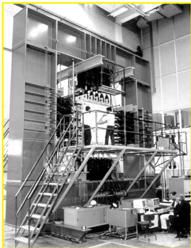
University of Toronto's Shell Element Tester
