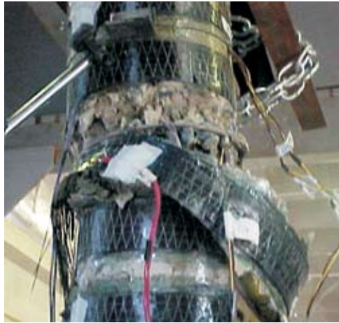
Figure 7 – Strap rupture – PC02S'5
