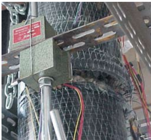
Figure 5 - Detail of rupture - PC01S'0
