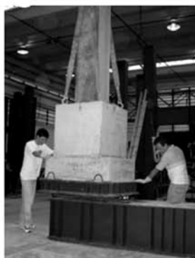
8 th ) Raising of specimen for reaction steel base
