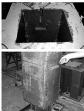
6 th ) Application of oil on socket base and column of specimens SI2 and SI3
