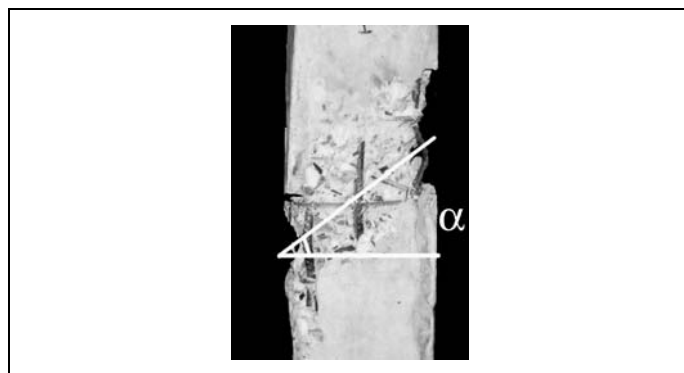
Figure 1 - Rupture shear plane.
