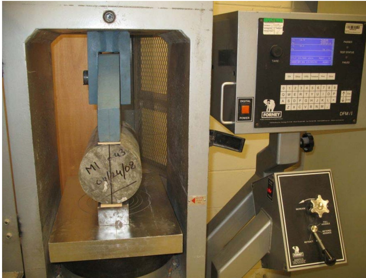
Splitting tensile strength test
