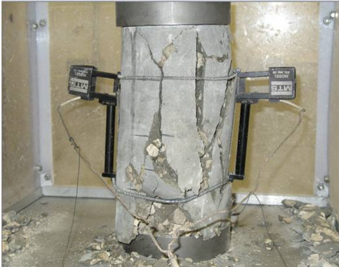
Compressive strength & elastic modulus test
